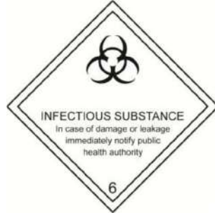
Figure A2. Hazard label for Category A infectious substances and for genetically modified microorganisms and organisms that meet the definition of an infectious substance, Category A
