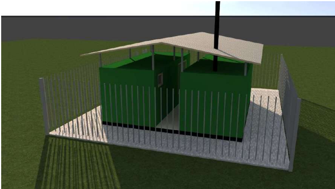
Figure 10: Proposed Containerised Incinerator to be installed at Levi Mwanawasa Hospital
